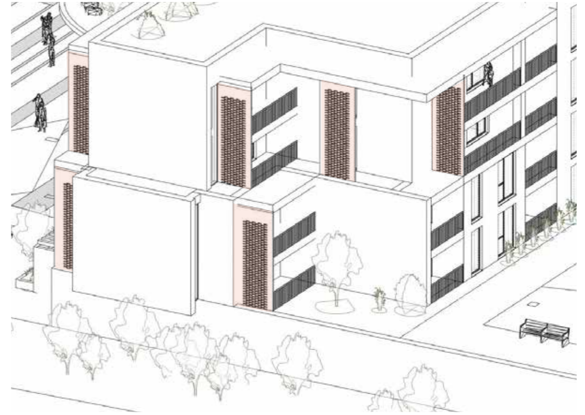
Hit and Miss brick details on southern facade
